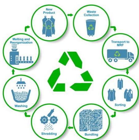
Figure 2. Plastic waste recycling process.
